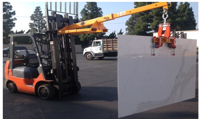
Example of forklift boom & pinch clamp
