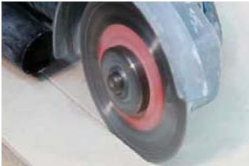
Example of variable speed grinder using diamond blade to make straight line cut out
